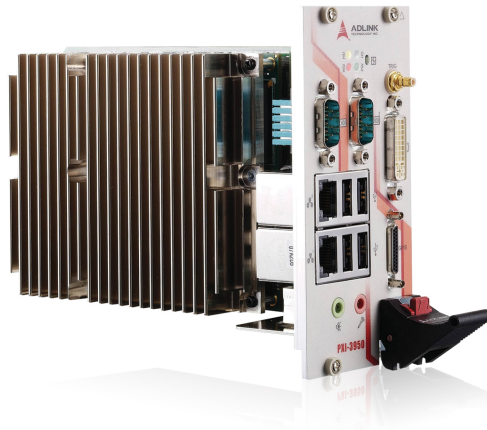
Figure 5. The ADLINK PXI-3950 Intel Core2 Duo T7500 2.2GHz PXI embedded controller.
